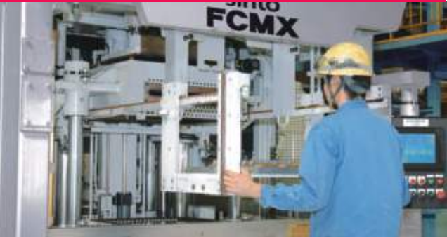
Matchplate is taken out quite easily by shifting to Pattern Change mode.
