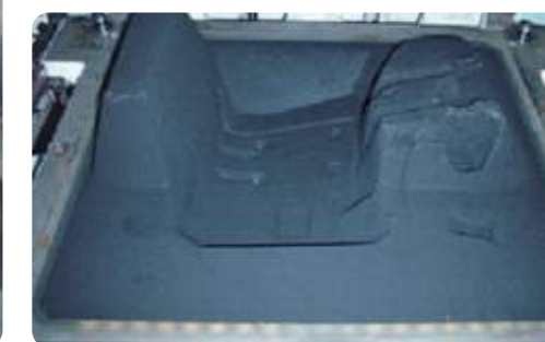
● Thin mold wall and deep cavity
