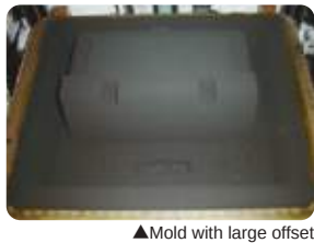
▲ Mold with large offset
