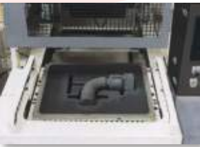
Drag mold slides out
