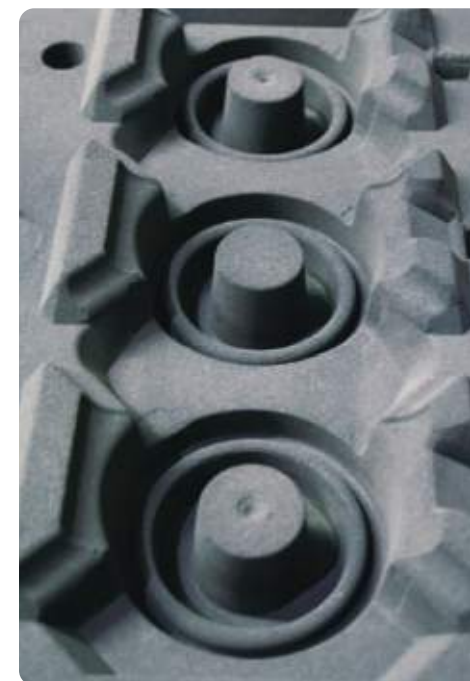
● Complicated pattern configurations with pockets
